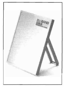
A flat Ku-band DBS antenna need only be about one foot square. Photo courtesy of Comsat and Matsushita.
